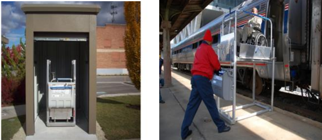
Figure 2. Wheelchair Lift in Protective Shed and In Use
