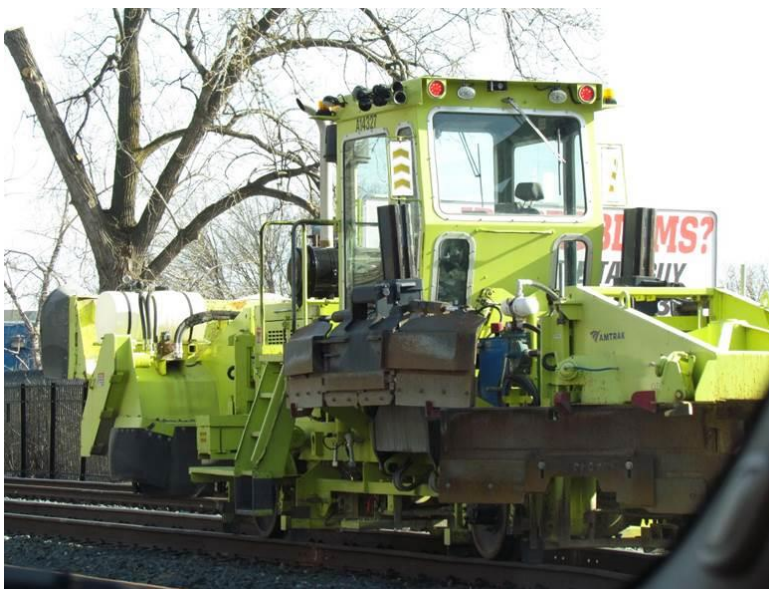
Figure 3. Ballast Regulator Used to Secure Rail for Albany Double Track
